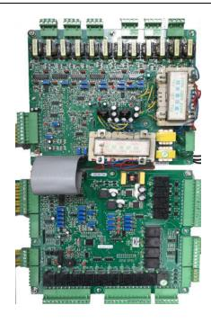
► Marstech is with DSP technology fully controlled. Charger is base on Thyristor + with Isolation transformer, Input PF >0.9, Low harmonic <5%, Standard low DC Ripple < 1% for 3 phase systems and Charger characteristic according DIN 41773 (UL)
